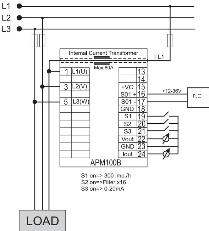
Typical connection between APM100B and PLC
